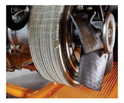
The HPP's efficient cooling system keeps out dirt and debris. Easy access allows cleaning of the radiator with a low pressure washer. (*Less than 500 psi.*)
