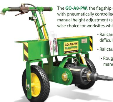
The **GO-A8-PW**, the flagship of our line, is an air-powered Gate Opener on a wheeled-cart with pneumatically controlled pivot wheels (follow traveling gate or moving train), and manual height adjustment (accommodate varied-height capstans). The GO-A8-PW is the wise choice for worksites which experience:
