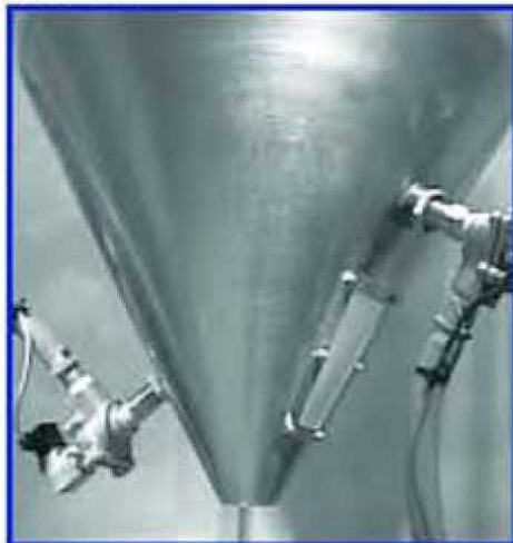
Stainless steel VA-06 Airsweeps keep batch hopper flowing.
